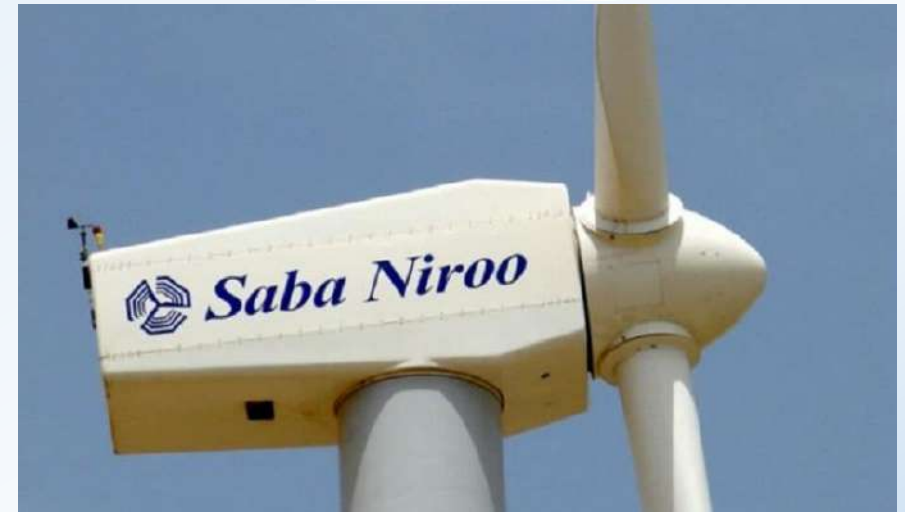
Wind Turbine 660 kW
